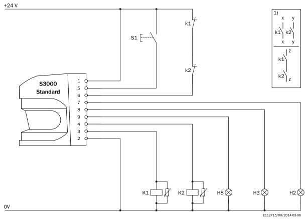
S3000 Standard in conjunction with relays/contactors
