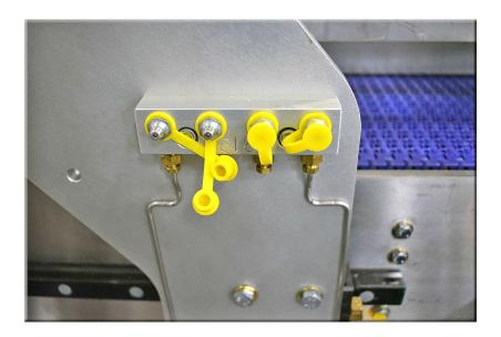
Grease zerks are color-coded to indicate frequency of manual lubrication.
