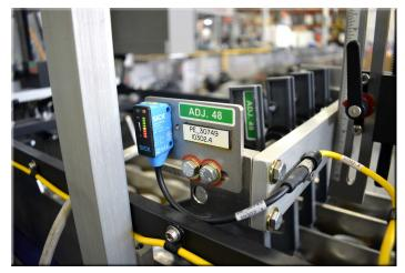
Right Angle Sufficient Surge Off Photosensor
