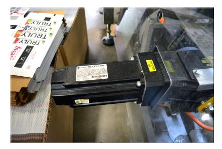
A servomotor is used in a closed-loop system that is capable of being precisely controlled. A resolver or encoder provides constant and highly accurate feedback of the motor's exact position, speed, and torque to the motor's servo drive (also called a controller). Through the drive, the PLC commands the servomotor to start, stop, and vary its speed and direction in accordance with the PLC program.
