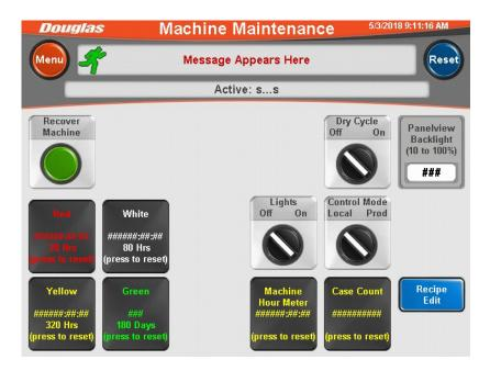
The **Recover Machine** button initiates machine recovery, which recovers the machine's servos to their proper positions.
