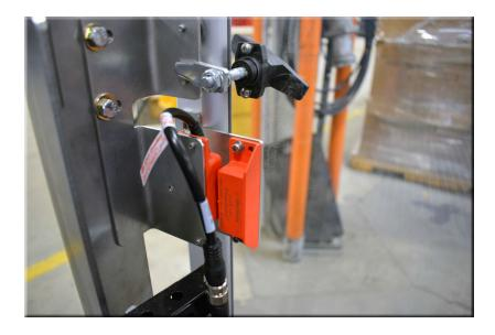
A magnetically coded guard door interlock switch is mounted on guard doors that may be opened without the use of a tool.
