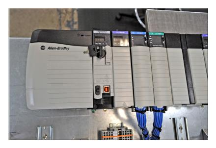
The PLC (Programmable Logic Controller) is a digital computer that controls machine operation.
