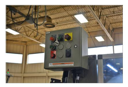
The **Panel Enable** button enables the auxiliary control panel. The operator cannot start the machine from this control panel unless the Panel Enable button is pressed and illuminated.
