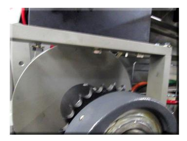
11. When re-installing, ensure that the hole pattern is opposite the sprocket side.
