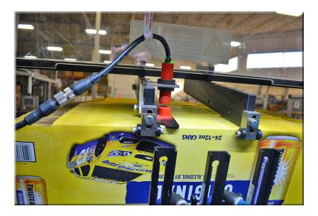
A magnetic magazine safety switch is mounted on the magazine, which controls two parallel contacts. The switch is connected in series to provide the machine with redundant circuits. The machine cannot run without blanks in the magazine.
