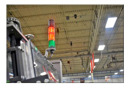
The stackable light column contains three lights and a horn to signal the operator of a machine condition.
