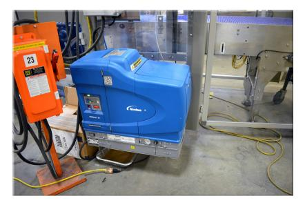
This machine uses a hot melt applicator. The melter liquefies solid-form hot melt and maintains the hot melt at the desired temperature. When the guns activate, the melter pumps the liquefied hot melt through the hoses and out the gun nozzles, where it is applied to the surface of the blank.
