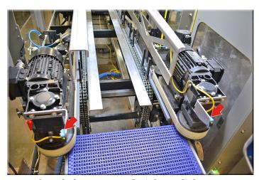
Left End Flap Open and Right End Flap Open Photosensors
