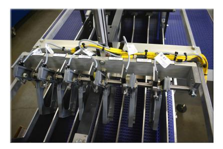
Proximity sensors are able to detect the presence of nearby objects without any physical contact. Proximity sensors detect the presence or absence of an object by emitting an electromagnetic or electrostatic field and looking for changes in the field.
