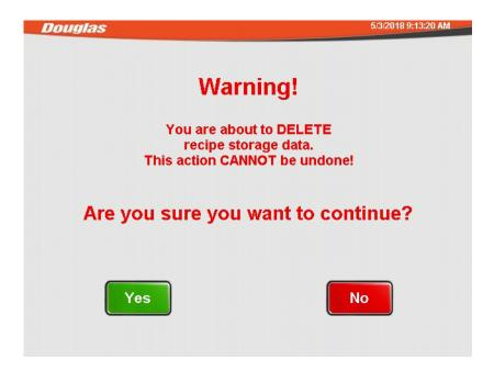
This screen will appear after the Delete Recipe button on the Recipe Control Screen is pressed.
