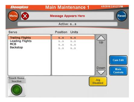
The current **Position** and **Units** are displayed for each **Servo** on this module. Press the **Up** or **Down** arrow buttons to scroll through the listed servos.
