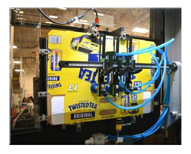
2. Adjust the magazine clips if necessary. Continue to load blanks until the magazine is full.
