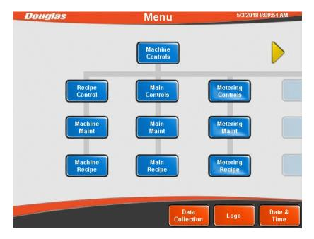
The Menu Screen allows the operator to navigate between screens. Press the desired screen button to advance to the corresponding screen.
