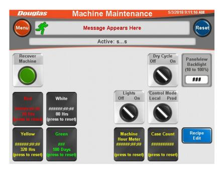
The **Recover Machine** button initiates machine recovery, which recovers the machine's servos to their proper positions.
