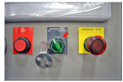
placed on the selector switch when lockout is desired. Set the selector switch back to No and then reset the machine to allow for restart.
