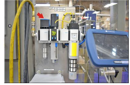
supply to the machine. To allow pneumatic pressure to return to the machine, turn the valve back to the shut position.
