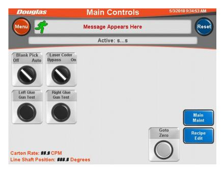
The **Blank Pick Off/Auto** selector switch disables or enables the blank pick vacuum.
