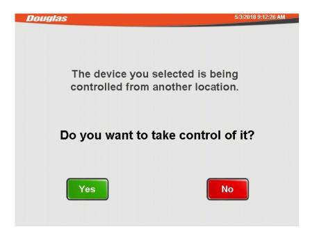
This screen allows personnel to take control of machine operation controlled from another location.
