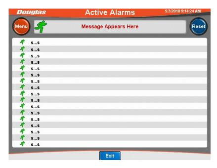
This screen displays currently active faults and alarms. It can be accessed by pressing the message display bar on any applicable screen.
