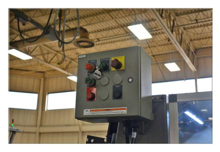
The **Panel Enable** button enables the auxiliary control panel. The operator cannot start the machine from this control panel unless the Panel Enable button is pressed and illuminated.
