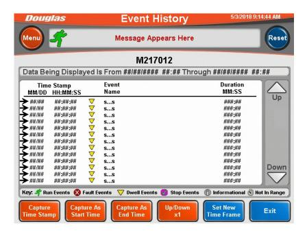
The **Data Being Displayed is From # Through #** display indicates the time frame of the displayed data. The percentages for selected data will appear when the Set Data Time Frame button on the Time Frame Setup Screen is pressed.
