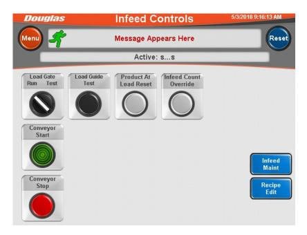
The **Load Gate Run/Test** selector switch, when set to Test, makes the **Load Guide Test** button appear.
