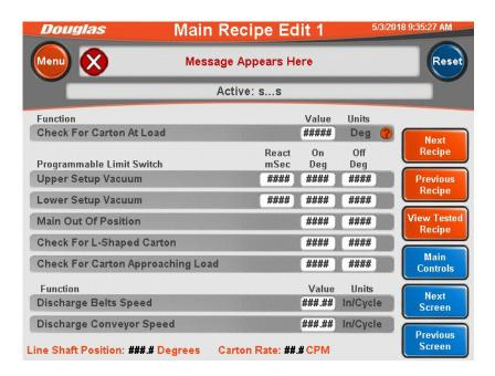
The **Recipe Display Bar** indicates the recipe to which the screen settings apply. An active or inactive display bar indicates the recipe status. The active recipe is the recipe the machine is currently running.
