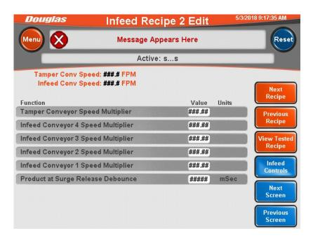
The **Recipe Display Bar** indicates the recipe to which the screen settings apply. An active or inactive display bar indicates the recipe status. The active recipe is the recipe the machine is currently running.
