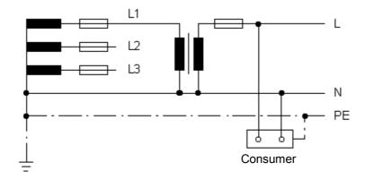
A transformer has to be provided on site in a TN-S network which supplies the necessary voltage of 230 V / 115 V as in the above diagram. The transformer can also be an autotransformer.
