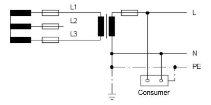
A transformer has to be used as in the above diagram. A TN-S network is then produced as from the transformer. A suitable earth has to be provided. It has to be checked on site whether such a network is permissible on site.
