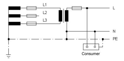
Directly connecting the HEUFT devices to two external conductors is not permissible if there is no neutral conductor available even if the voltage is within the specified voltage limits. A transformer has to be used as in the above diagram.
