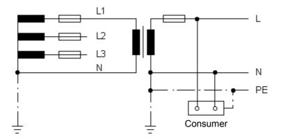
TT networks have a neutral conductor but the PE conductor is not run separately in the system. A transformer has to be used as in the above diagram. A TN-S network is then produced as from the transformer. Other possible options are disapproved of for safety reasons.
