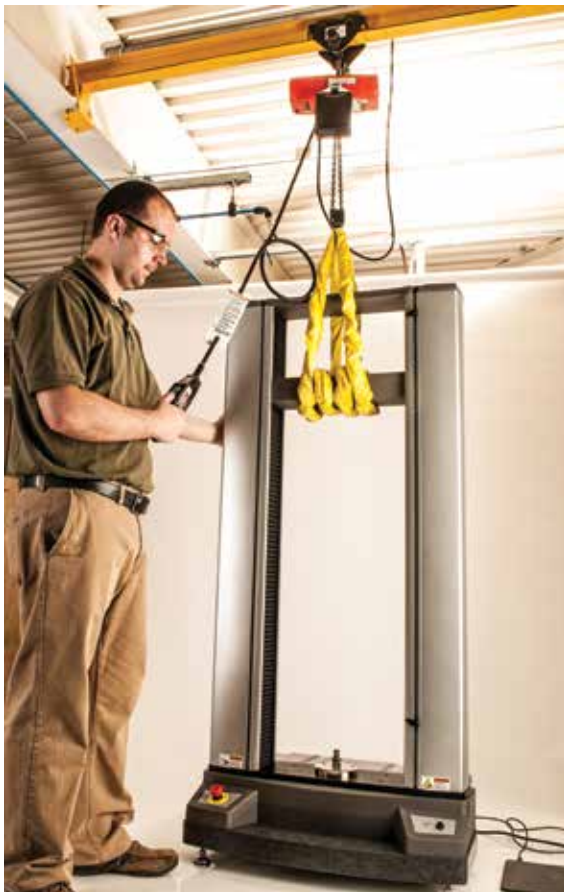
Lift by Crosshead Do NOT lift by top plate
