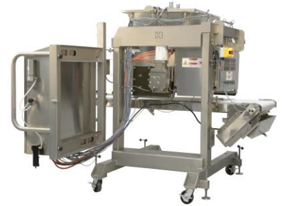
SWING-OUT ENCLOSURE ON ROBUST FRAME
