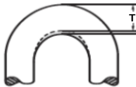
Minimum Allowable Chain Link Thickness at Any Point
