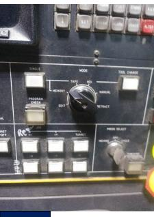
Go back to control panel, turn selector switch to manual.
