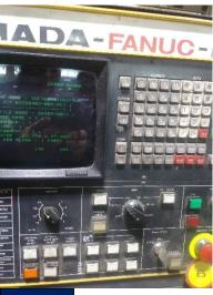
Delete old order that has been completed (ex. O#####). Put in new order (ex. O####) Press Read button, (will be blinking)
