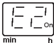
Fig. 24 Display of the malfunction E2, failure to build pressure at the end of the line.
