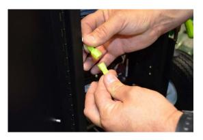
2. CONNECT THE UPS FUSE. FUSE IS LOCATED IN ENVELOPE. PLUG UNIT IN TO EXTERNAL POWER AND TURN UNIT 'ON'.
