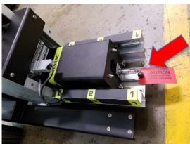
7) Next carefully allow the motor carriage to spring forward to it normal resting position as shown in picture to the right.
